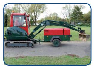
When leaving equipment overnight on sites, secure small portable equipment under the boom arms of mini-excavators, then use immobilisers or hydraulic locks to prevent removal
