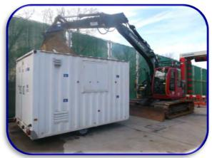
To make it difficult for criminals to break in to your portable store, we suggest positioning a machine in this manner. This will not only make it difficult to break into the store but will stop the store from being lifted.
